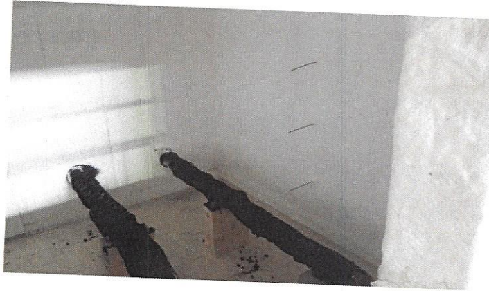
Figure 3. Propane Burners and Room Thermocouples.
